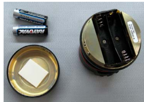
Figure 13. Accessing and replacing the batteries.
