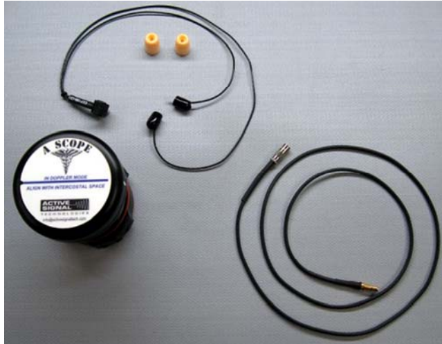
Figure 6. Doppler returns are best heard using in-ear ear buds or CEPs combined with a circum-aural hearing protector or a helmet with integrated hearing protection.
