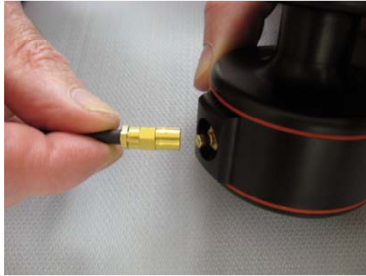
Figure 2. Connecting the headset cable.
